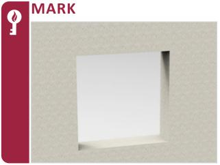
Mark out and cut an opening in the ceiling or wall to suit the dimensions of the access panel (eg. 450x450mm), taking into account the position of existing joists.
